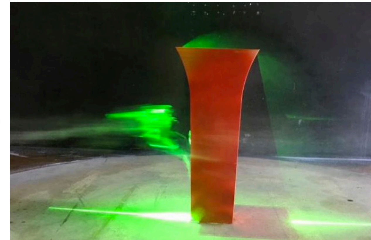
Smoke testing of a building with a tapering shape (the direction of air inflow is marked with an arrow)
